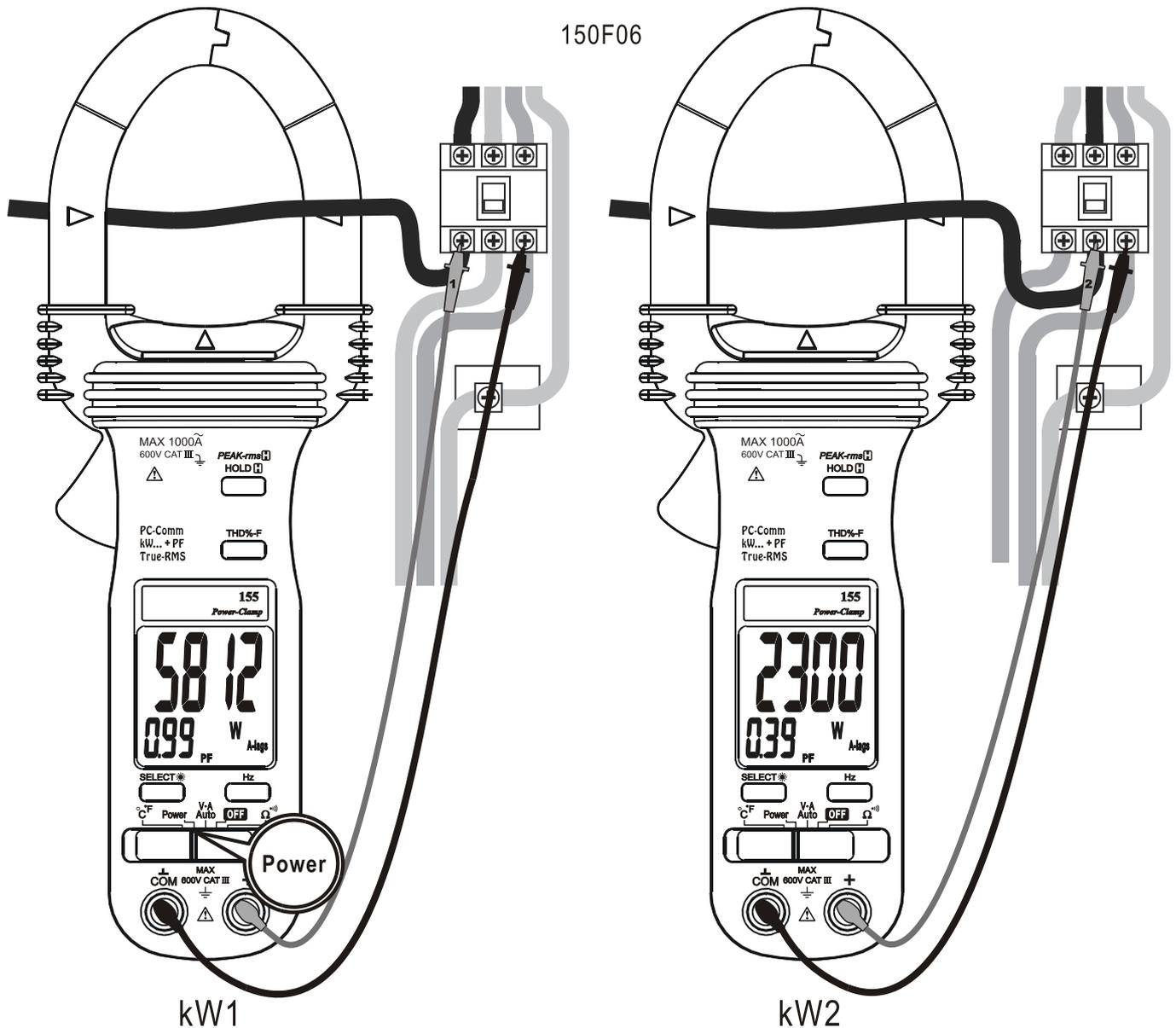
In both un-balanced and balanced load cases, 3-Phase 3-Wire (3~3W) systems, measure the power components  $kW_1$  and  $kW_2$  separately as illustrated. System (total) power  $kW_{Total}$  is the summation of the two measured power components. That is:
