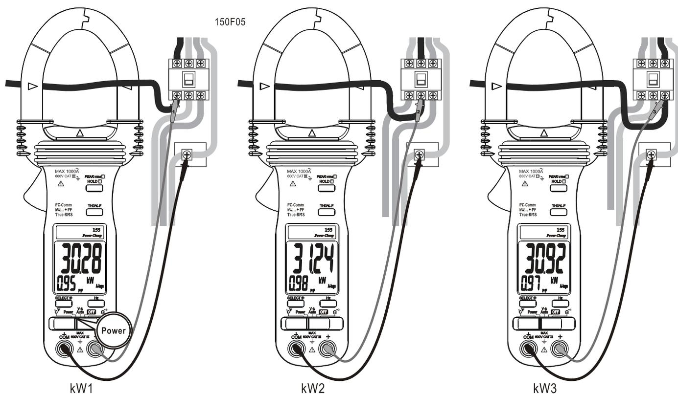
In both un-balanced and balanced load cases, 3-Phase 4-Wire (3~4W) systems, measure the phase-to-neutral powers  $kW_1$ ,  $kW_2$  and  $kW_3$  of each phase separately as illustrated. System (total) power  $kW_{Total}$  is the summation of all three phase-to-neutral powers. That is:
