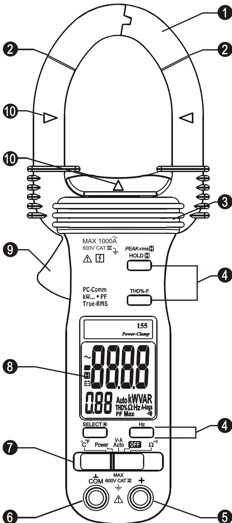
1) Transformer Clamp Jaws for AC current magnetic field pick up
